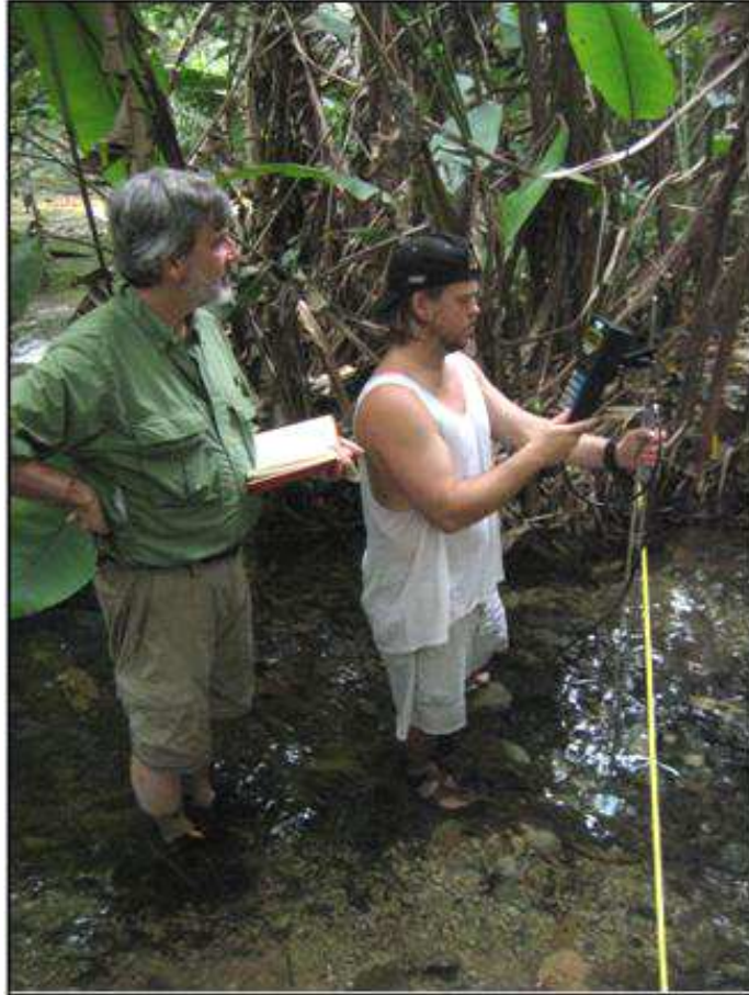
Figure 4. Dr. Christopher Duffy and Kirk French gauge the Picota Stream with the SonTek FlowTracker.
