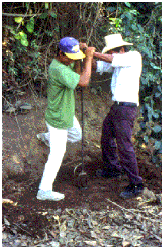
Figure 6: Enrique Urisas and Leonel Urisas demonstrate the use of a bucket auger for obtaining clay samples.
